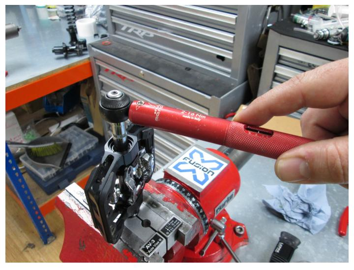
Place the body back over the axle and re-install the retaining nut and wash that secure the axle in the cleat body. Using your 8mm socket, torque this to 10-13Nm remembering AGAIN that the RH axle uses a LH thread so please make sure you are tightening in the correct direction.
