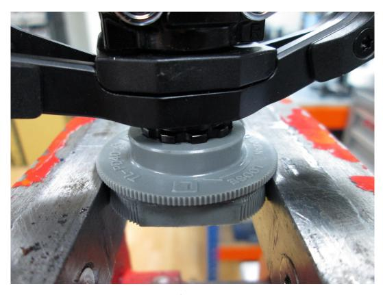
Using your Shimano TL-PD40 remove the fastener that secures the cleat body to the cage.
