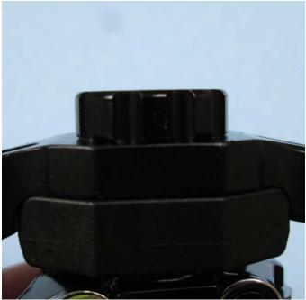
Apply a light covering of thick grease to the load surface of the cleat body fastener and the pedal cage that the fastener contacts. Thread the fastener back into the cleat body (hand tight) remembering that the <a href="https://example.com/remails/remails/">RH PEDAL USES A LH FASTENER.</a>
