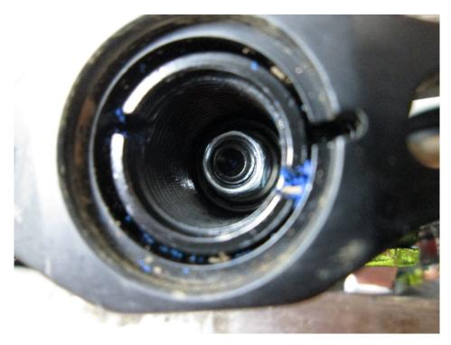
This will expose the axle nut. Remove the nut to free the axle.
