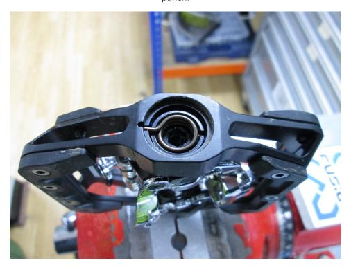
Remove your end cap with the 3mm Allen key and remove the spring.
