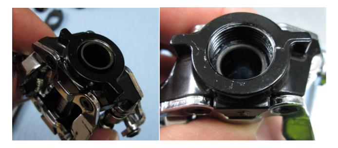
Thoroughly clean the cleat body inside and out. Apply a thin layer of Loctite 641 bearing retainer around the bushing and press into the cleat body. The bushing has a 'leading' edge which is chamfered, make sure this end of the bushing is inserted into the body first.
