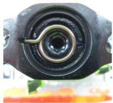
Install the 6mm end float nut to 15Nm (Standard RH Thread), align the pedal cage spring keys with the corresponding cleat keys and fit the spring.
