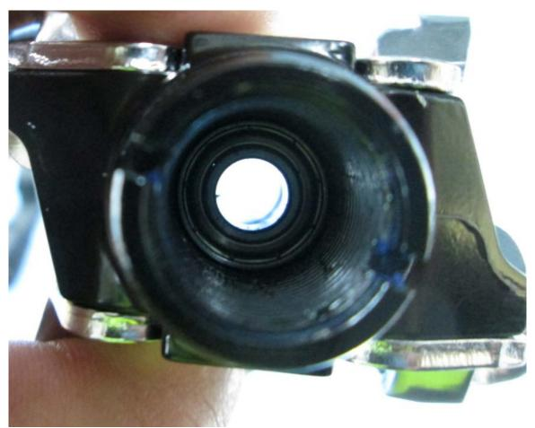
Next, use your punch to seat the cartridge bearing into the cleat body.
