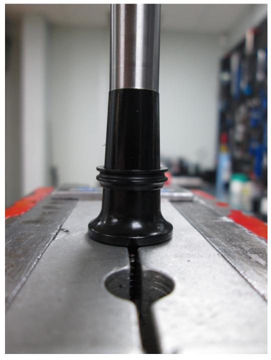
Slide your new dust seal over the axle making sure that the chamfered end points toward the axle threads (away from the pedal.
