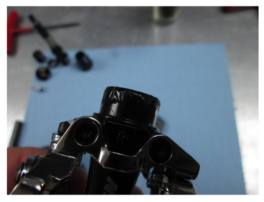
Apply a thin layer of the thick grease to the cleat body that contacts the pedal cage.
