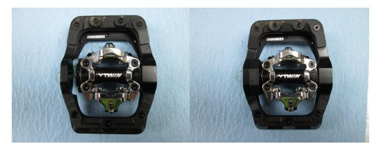
Slide the cleat body back into the pedal cage and insert the anti-rotation bumper.
