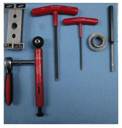
**Tools Needed:**  $8 \text{mm } \frac{1}{4}$ " Drive Deep Socket, 6 mm & 3 mm Allen Keys, Shimano TL-PD40 Tool, Axle Vice & a small deep punch.
