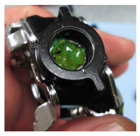
Use a generous amount of thick grease to cover the bushing load surface.
