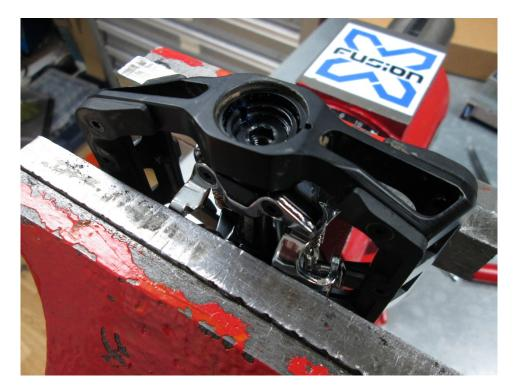
Next, grip the cleat body in a vice to remove the end float nut with the 6mm Allen key.
