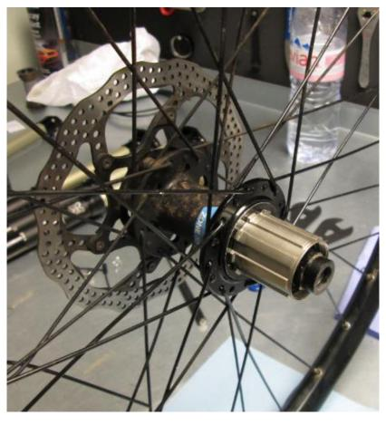
Thread on your drive side end cap and torque both caps to 10-13Nm. That's it your all done and have a fully service Zone rear hub.
