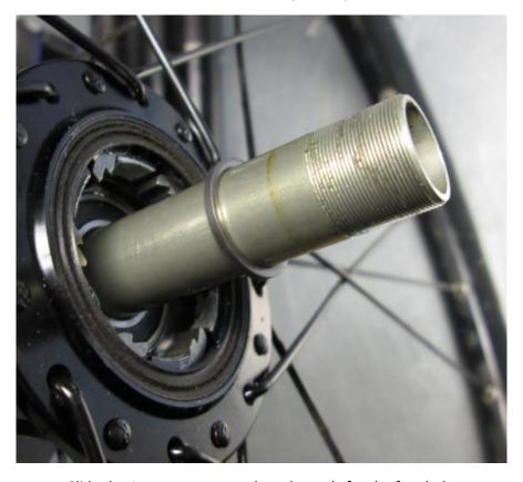
Slide the 1mm spacer onto the axle ready for the free hub.
