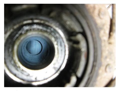
Once you have pulled the free hub and axle you will need to push the spacer tube over to create a secure punch surface, I use the punch to just slide it over a touch.
