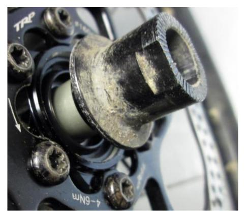
Drift the non-drive assembly into the hub making sure that the seal is seated correctly, pull the axle just to make sure it's all seated perfectly.
