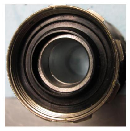
Clean up the dust seal and press into the seat in the free hub body, and that's the free hub finished.
