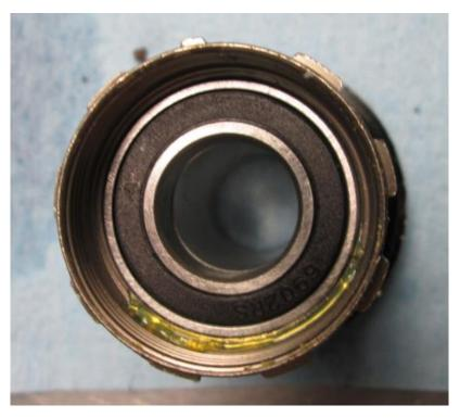
For the next part an arbour press is preferred but not everybody has one. Press the 15268-2rs bearing into the Inboard position then place your spacer tube in the body and press the other 15268 bearing in the outboard position, making sure the spacer tube is not at an awkward angle.
