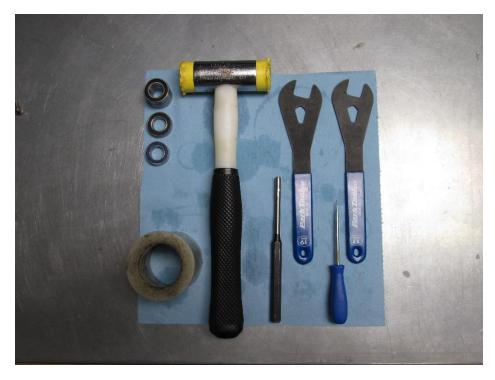
**Tools needed:** Hub Support, Soft blow nylon mallet, punch (not a screwdriver), 17mm &19mm cone spanners, a dental pick.
