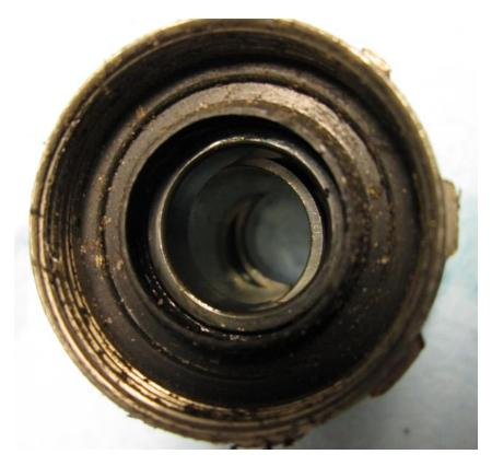
Next onto the free hub, use the same process as the hub body and move the spacer to the side and use your punch to drift them out.
