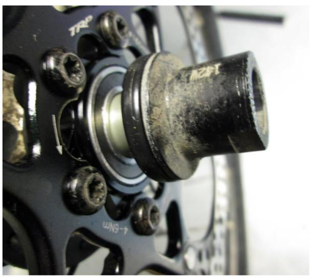
Slide the assembly through the hub and into the drive side bearings.
