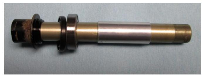
Thread you non drive side end cap on the axle, slide the dust seal on, apply a small amount of grease on the axle and slide the bearing and spacer tube on.
