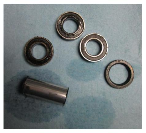
Once you have punched the non-drive bearing through you will have plenty of access to the 1x 15267 bearing on the drive side, you will in total have 2x 15267 bearings, non-drive seal & the spacer tube.
