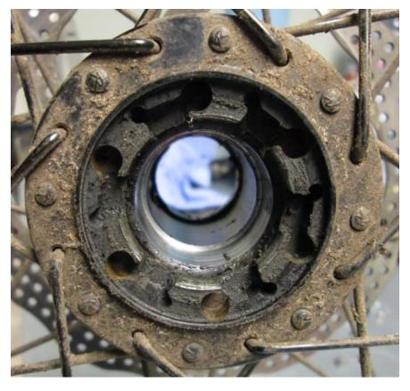
Once you have removed the pawls and springs, give the hub a good clean to remove any dirt, grime & debris.
