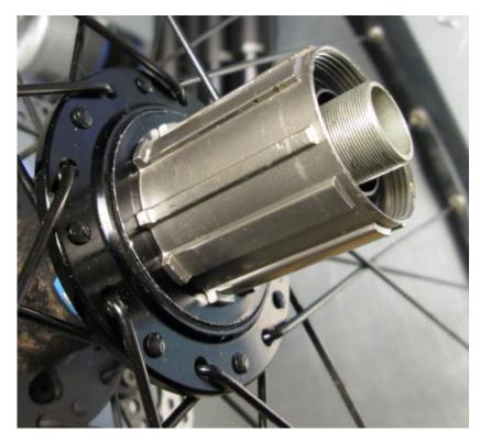
Slide the free hub onto the axle, lightly grease the ratchet ring on the free hub before installing.
