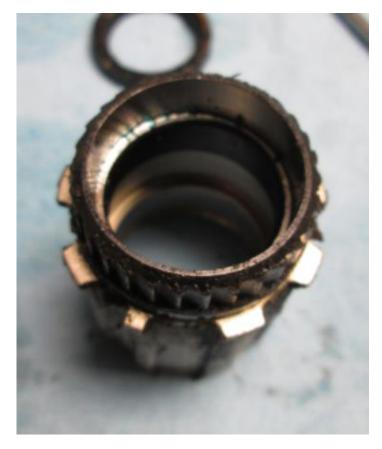
Leaving you with the bare shell and the old 15268-2rs x2 bearings and the spacer tube.
