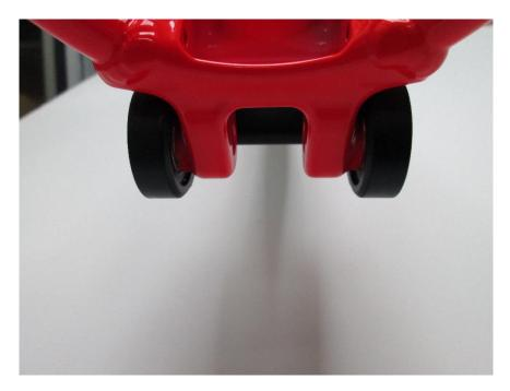
Now you have the link fully pressed over the bearings you can torque the lower link bolts to 15-18Nm and the 8 x 3mm link spacer bolts to 5-8Nm.
