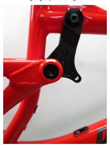
Start by removing your shock from the frame. If you're are dealing with a complete bicycle, remove the Crank, Chain & rear wheel to make sure you have the room to work on the frame.
