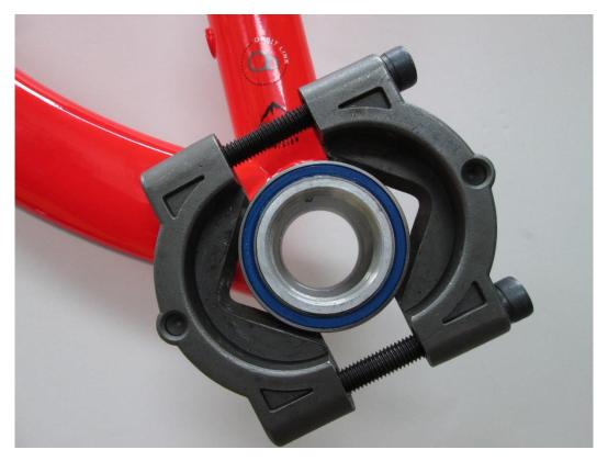
Use a crown race puller. This is the most efficient and least damaging way that we have found that will remove the bearing nice and square and runs no risk of damaging the frame.
