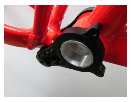
Now onto the lower link. Remove the 6mm and 3mm bolts on the D/S Link plate.
