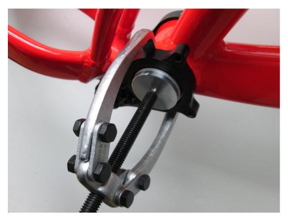
Place your SLED BB plug (DMR-TOOL-BEARING-SUPPORT) into the BB shell and use your gear puller to hook onto the link plate being careful to not catch the frame, pic below.
