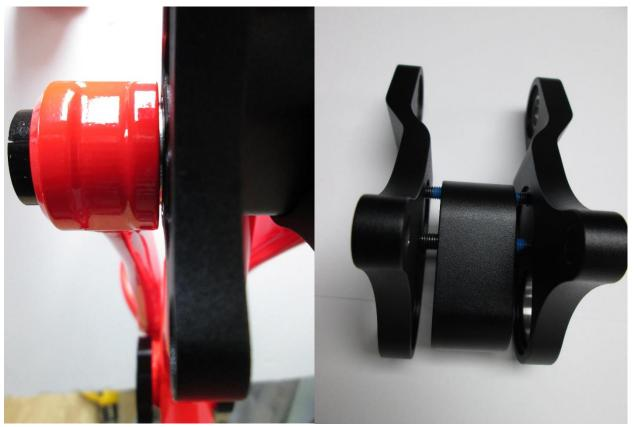
As you remove the collet be aware that there a 2x washers (DMR-S-SLED-WASHERS) that can easily be lost as you pull the collet from the frame. After the collet has been removed, undo (don't remove) the 6x 3mm bolts from the centre of the link plates. Then you can remove the 2x 6mm bolts (DMR-S-SLED-LINK-BOLT) that attach the upper link to the top tube, the link is now free from the frame to service.
