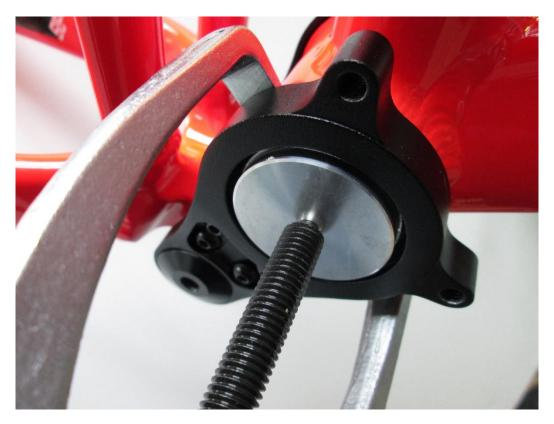
Gently wind the gear puller to remove the link plate. Hopefully when you remove the link plate it will take the bearing off the BB shell with it but if it doesn't, he is our suggestion...
