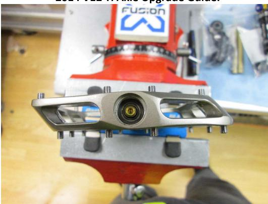
Slide the body back over the axle gently and make sure the axle is protruding through the cartridge bearing.
