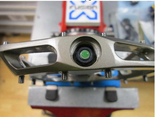
Remove the 9mm nut (RH Pedal has a silver LH thread nut).
