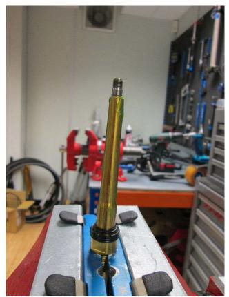
Apply grease to new axle making sure the bushing contact patch has a thin layer of grease around it.
