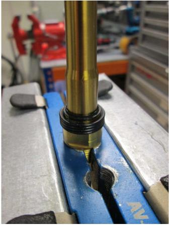
Slide the 2 rubber seals onto the new Ti Axle.
