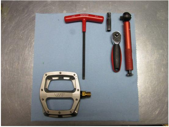
Tools needed: 6mm Allen Key, 9mm ¼ inch socket, ¼ inch Ratchet, ¼ inch Torque Wrench.
