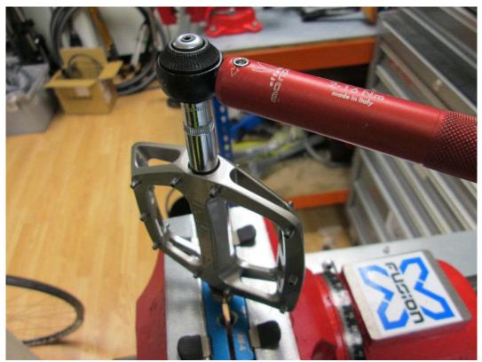
Thread the 9mm nut back onto the axle and torque to 10Nm maximum.
