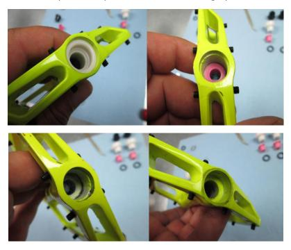
Next using a broad punch, lightly drive the bushings out of each end of the pedal body and clean bushing seats thoroughly.
