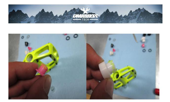
Replace the bushings for your nice new ones from your service kit and press into the pedal body with plenty of grease. The bushings should press in easily by hand, if a bit tight don't be afraid to help them home with your punch and nylon mallet.
