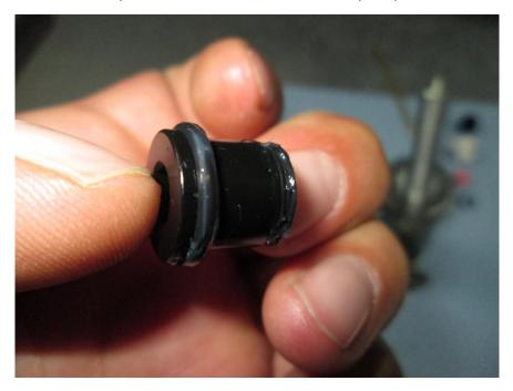
Install the x-ring onto your end nut and cover with liberal amounts of grease.
