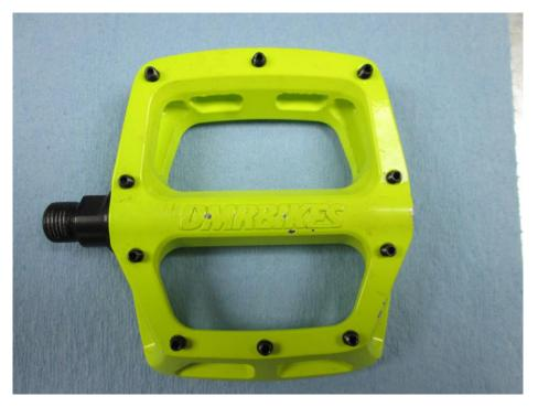
There you have it, a fully service V8 pedal. **Parts Used:** DMR 2016 V8 Service Kit – DMR-S8-KIT-V2
