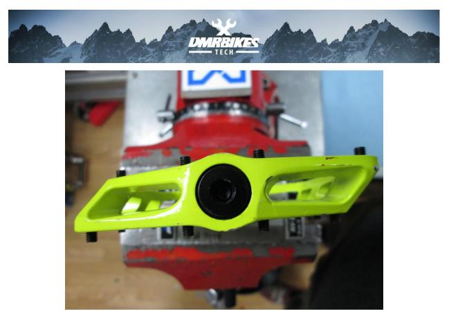
Re-fit the end nut and torque to 8-10Nm
