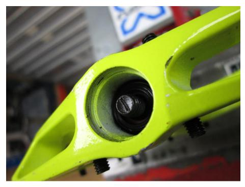
Remove end nut to free the pedal body. Clean the axle thoroughly and check for imperfections.
