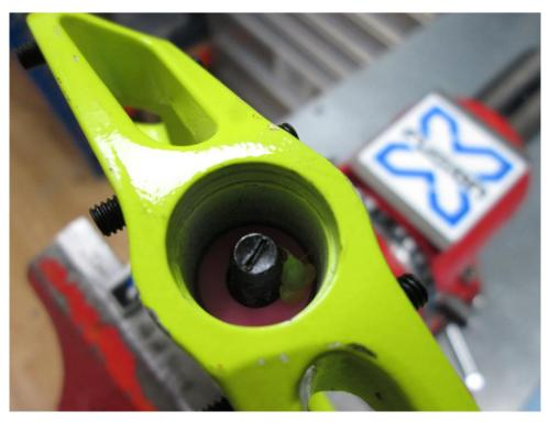
Grease your axle well and slide the pedal body back in place.
