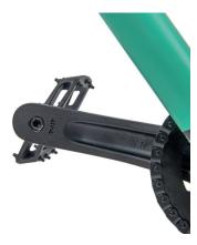
Tighten each pedal up using the allen head on the inside of the axle.
