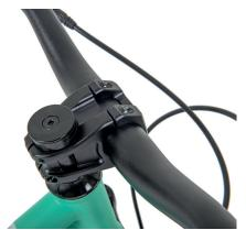
To tighten the headset you need to make sure the stem is loose on your steerer (the two bolts towards the back of the stem). Once these are undone you can tighten you headset preload on the top cap of your stem. Once your headset has no forwards/backwards movement and remains easy to turn left to right you are ready to tighten the stem/steerer bolts towards the back of the stem. Make sure you tighten these to the reccomended torque. See Table 1
