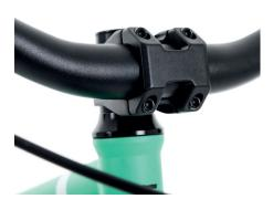
Bar clamps should be fastened seperately. Torque figures can be found on the previous page or see Table 1.
