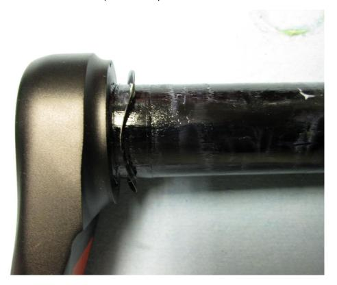
Slide the wavy washer over the axle all the way against the LH crank arm.
