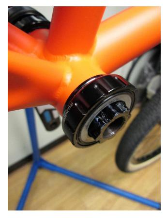
Slide the crank through the BB until the axle meets resistance on the RH BB cup.
