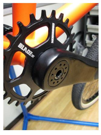
Thread the RH crank arm on, making sure you have aligned the splines correctly then torque the arm to 48-55Nm.
