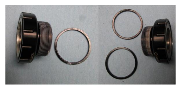
For a 68mm BB shell add 1 spacer to the LH cup and 2 spacers to the RH cup.
