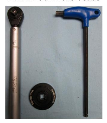
Tools Needed: 10-40Nm 3/8" Torque Wrench, 8mm Allen Key & Praxis M30 BB tool
