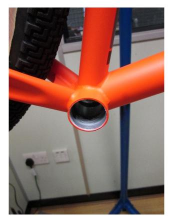
Apply a liberal amount of Anti-seize grease or Copper slip grease to the BB threads.
