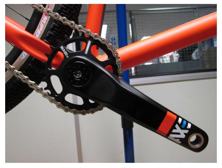
There you have it, a correctly installed DMR AXE Crank.
